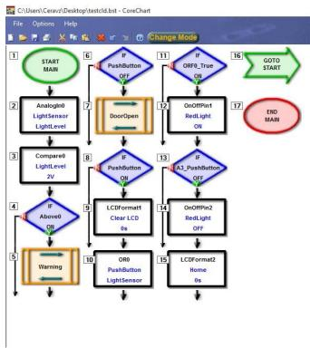
Figure 6: The complete alarm system
