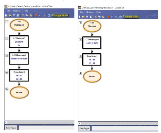
Figure 7: The subroutines for the complete alarm system
